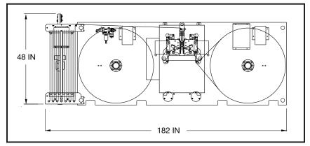
As with all Martin products, the NCHW is application-engineered to your process. Current web widths are to 24 inches (610MM) with splicing speeds of 1312 FPM (400 MPM) (based on roll weight and material splicing tension required). Contact Martin Automatic Inc for information.
