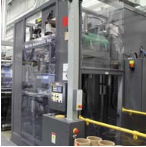
A Martin LRD Automatic Transfer Rewinder enables the Goss Vpak press to run roll-to-roll without stopping.
